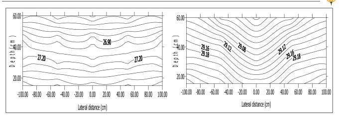
Fig. 1(b): Soil moisture distribution in micro sprinkler treated plot before and after irrigation
