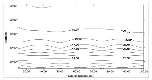
Fig. 1(c): Soil moisture distribution in control plot after irrigation
