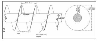
Fig. 1: Screw flight designed over the shaft
