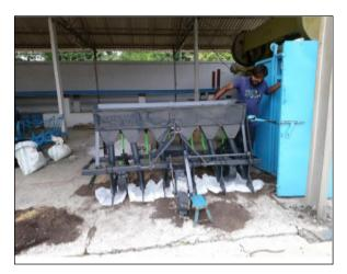
Fig. 2: Laboratory calibration of screw conveyor mechanism
