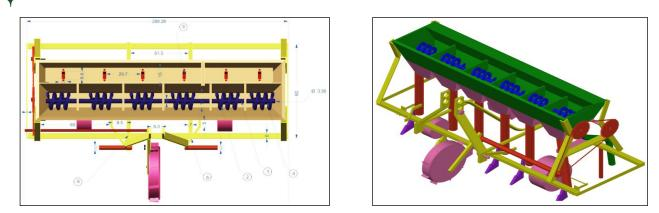
Fig. 4: Top view and perspective view tractor operated manure and seed applicator
