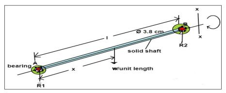
Fig. 7: Load distribution on the shaft
