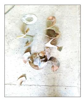
Fig. 6: Design of washer web for screw flight
