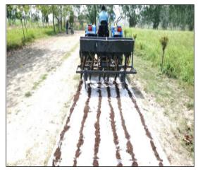
Fig. 3: Field performance test of screw convey or mechanism
