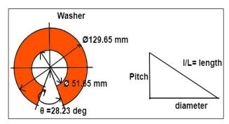
Fig. 5: Design of washer size to be select for developed screw flight
