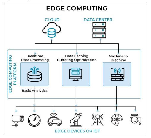
Fig. 1: Basic structure of Edge Computing in IoT Context
