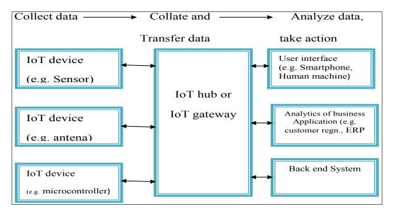
Fig. 4: An example of how an IoT system works from collecting data to taking action<sup>(17)</sup>
